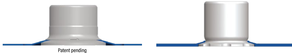
Standoff for sheets as thin as 0.1 mm
